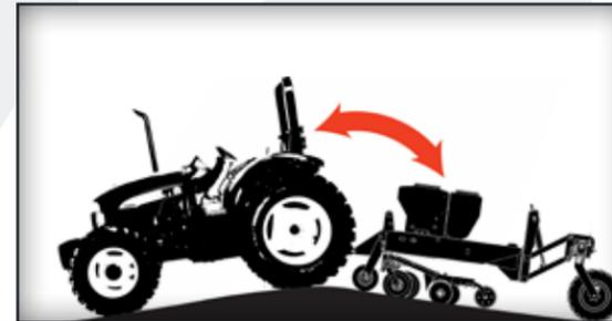
Two standard lift-assist wheels in the rear of the 3P806NT & 3P1006NT provide greater lift capacity and assist the tractor's 3-point. Straddle axle caster wheels provide maneuverability and strength.
