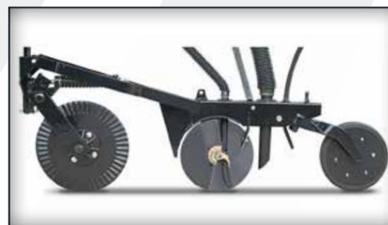
The O6 Series Row Unit by Great Plains utilizes the "Fluff and Plant" no-till system with an integrally mounted coulter to cut residue and prepare a mini-seedbed for the trailing double disc opener. Opener discs are 13.5" (34cm) in diameter with 4mm thick blades, 205 triple-lip sealed bearings, and 1/4" (19mm) opener disc lead.
