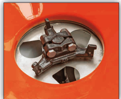
Agitator ensures even feed of the fertiliser
