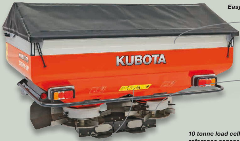
Three options of hopper capacity 1,100 – 1,550 – 2,000 litres
