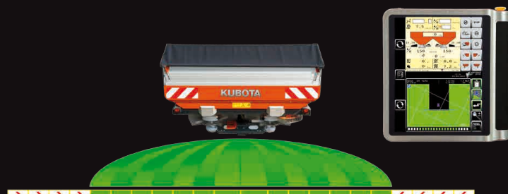
Decreasing the spreading width on both sides by 8m
