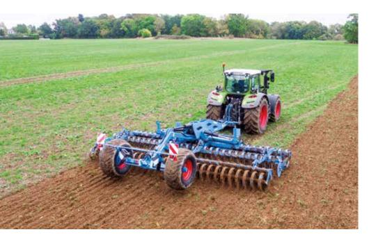
The Heliodor compact disc harrow from LEMKEN uses two rows of discs individually mounted to leaf springs. This system provides a uniform cultivation depth, whilst allowing individual discs to ride over stones when necessary. During stubble cultivation the discs ensure soil and vegetation are evenly and intensively mixed.
