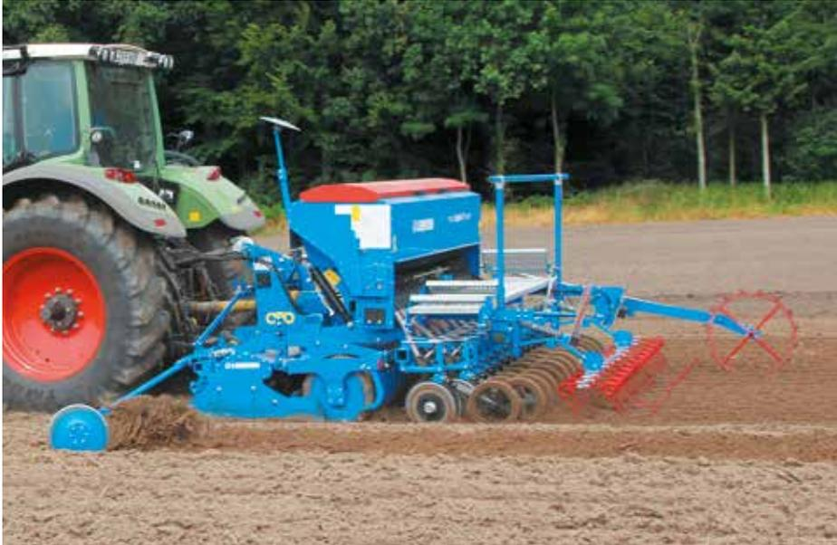
It is becoming ever more important to adjust the intensity of the seedbed preparation to the prevailing field conditions. Practice shows that the power harrow is a very versatile and efficient device and therefore best performs this preparatory task.
