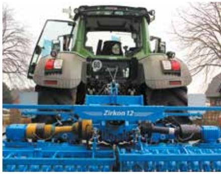
**Each PTO shaft with overload safety device**
