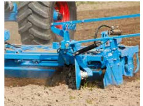
**Feed discs for precisely harrowed paths**
