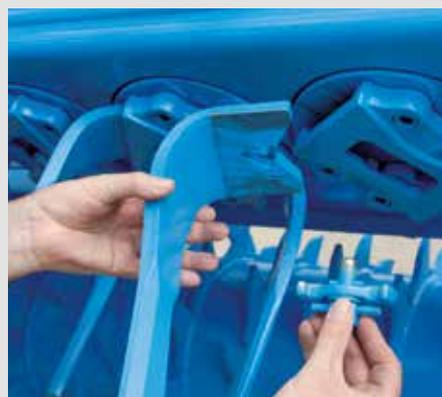
**Replacing a quick-change tine**
