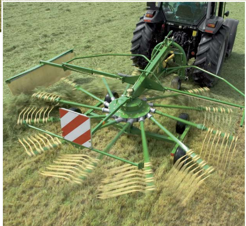
Perfect in work: using up to 13 tangentially arranged tine arms, the SWADRO 35 to 46 single rotor rakes deposit the crop in clean, even swaths.
