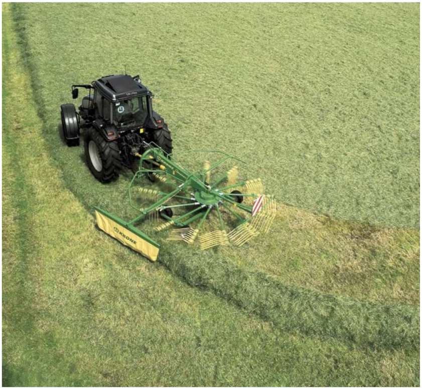
Tracks true: In any curve KRON Swadro single rotor rakes always follow the tractor.
