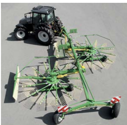
Agile through and through: the Swadro 807, 809 and 810 rake up everything due to their high maneuverability, even in restricted areas. With a wide wheel track on the running gear and a steering axle, they can master any corner.
