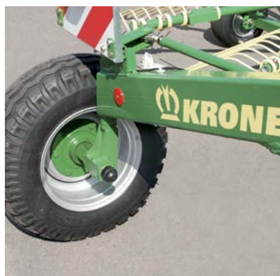
Optimally equipped: the large 10.0/75-15.3 8 PR tires and track-following linkage ensure absolutely smooth and stable travelling – an advantage when working on slopes or at high driving speeds.
