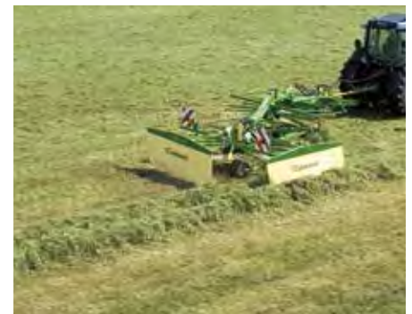
Forming double windrows Raking 12.40 m (40'8") into one double windrow
