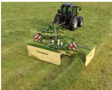
Forming one single windrow Raking 6.20 m (20'4") into one windrow
