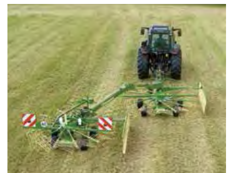
Forming double windrows Raking 12.40 m (40'8") into one double windrow
