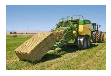
The VFS principle relies on a system of packer and feeder rakes, which feed the material into the pre-compression chamber where it builds up to receive an initial compression. After this pre-compression chamber is packed to capacity, the feeder rake feeds the material into the baling chamber.
