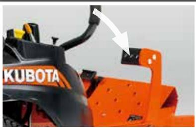
**1** Push and release the pedal to raise the deck
