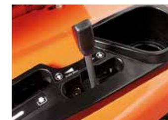
Hydraulic mower lift lever
