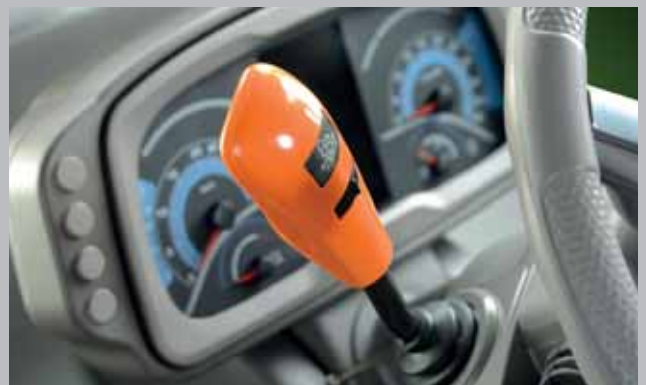
The direction of driving can be reversed with the individually adjustable powershuttle lever to the left of the steering wheel.
