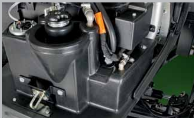
The fuel tank integrated into the front axle support can be filled even with the bonnet closed, while the auxiliary tank is located underneath the chassis.
