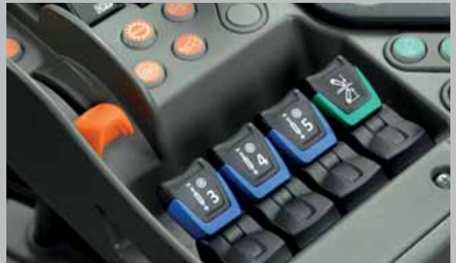
The activation of the front axle suspension is easy to access in the MaxCom control panel.
