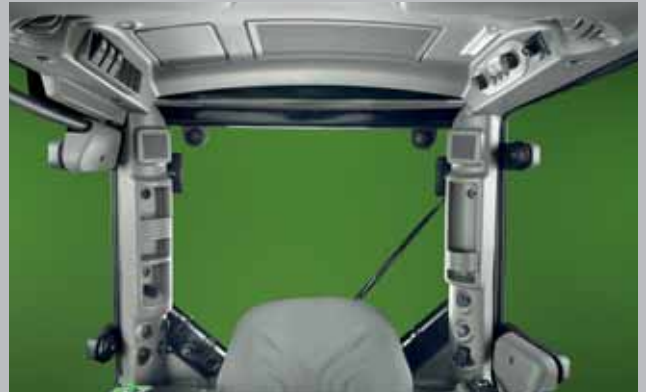
The air conditioning controls are easy to access on a display in the roof of the cab.
