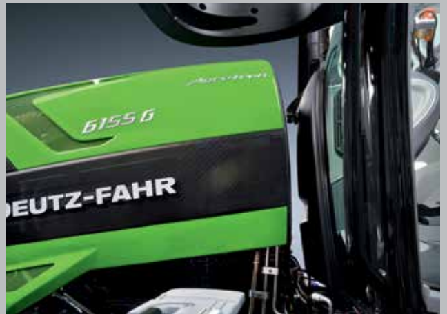
No connection between cab and engine hood - improved driver comfort with lower noise.
