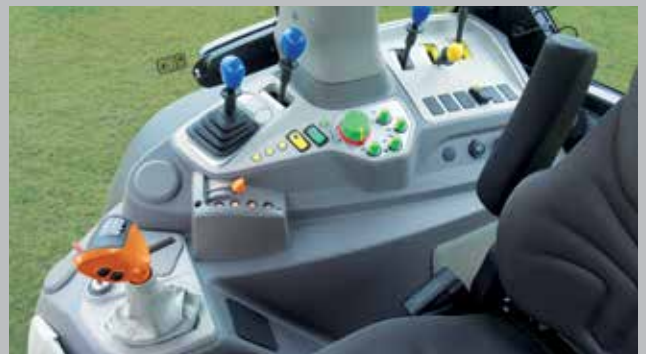
Powershift transmission layout
