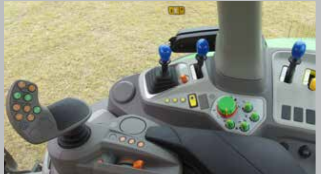
RC-Shift transmission layout
