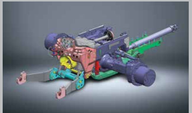
Electronic adaptive suspension incorporating an Anti-Dive and Anti-Rise system. The suspension can be used in the field and on the road. Fully lockable when needed.
