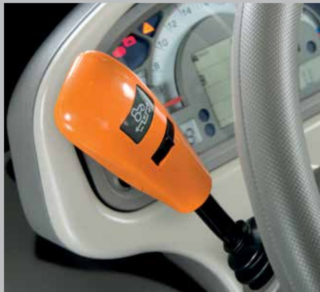
Modulation on Powershuttle lever with 5 adjustable settings
