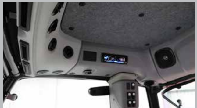
Air vents located throughout cabin.
