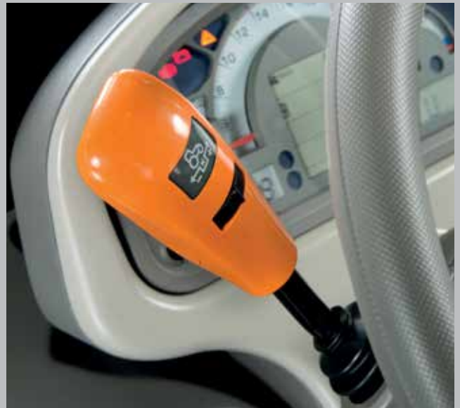
Modulation on Powershuttle lever with 5 adjustable settings
