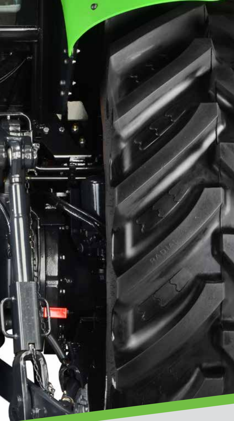
External rear lift and PTO remote controls
