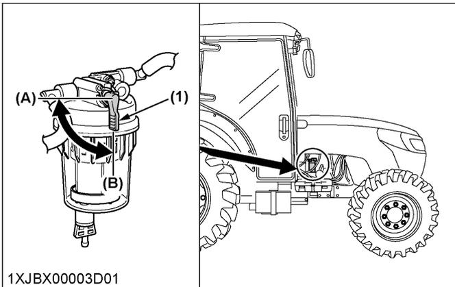
(1) Fuel shutoff-valve (A) "CLOSE" (B) "OPEN"
