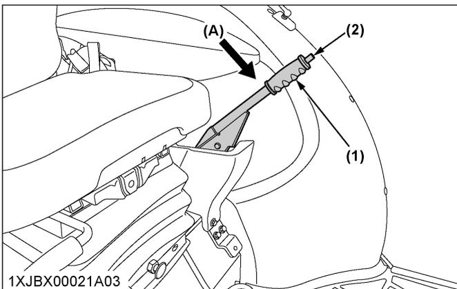
(1) Parking brake lever (A) “Push down to transport position”
