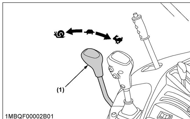
(1) Range gear shift lever
