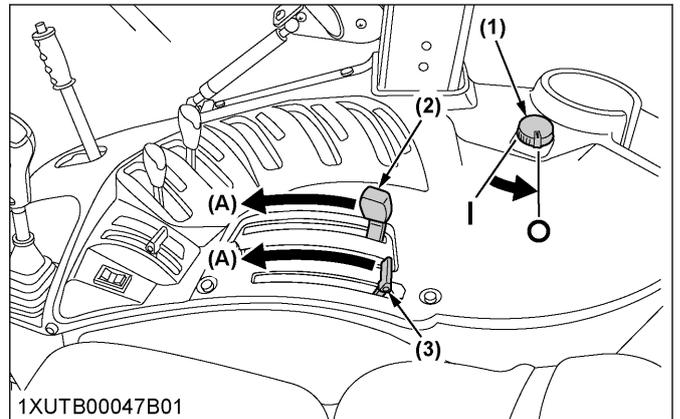
(1) PTO clutch control switch (2) Position control lever (3) Draft control lever
