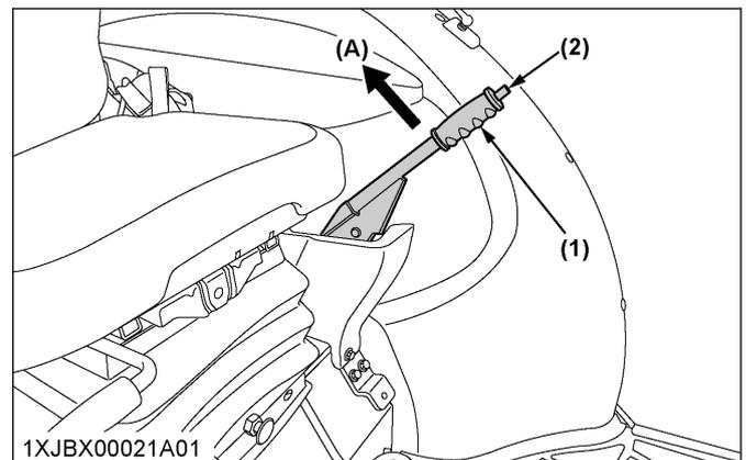
(1) Parking brake lever (A) “Pull up to parking position”
