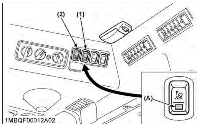
(1) Front work light switch (A) Indicator for work lights
