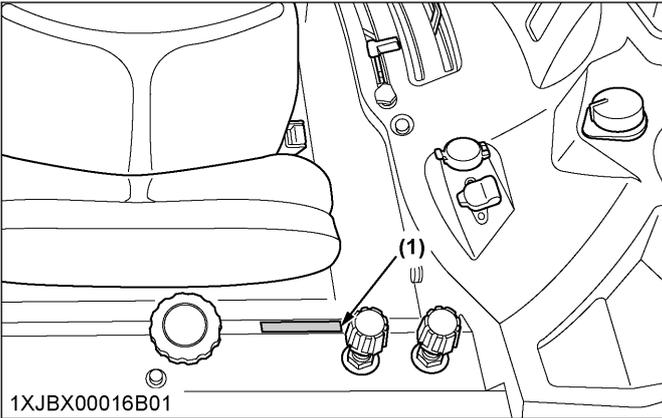
(1) CAB identification plate (CAB serial No.)
