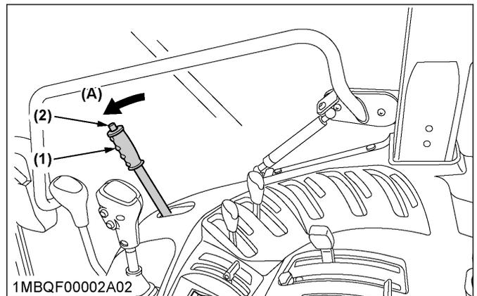
(1) Gear-locked parking brake lever (A) “Push to transport position”
