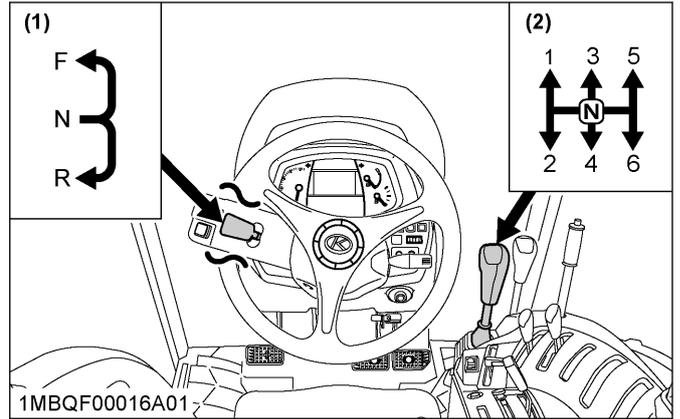
(1) Hydraulic-shuttle shift lever (F) "FORWARD" (2) Main gear shift lever (N) "NEUTRAL POSITION" (R) "REVERSE"
