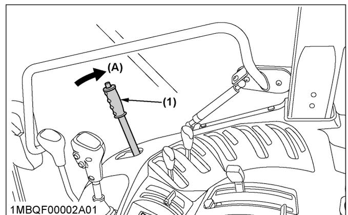
(1) Gear-locked parking brake lever (A) “Pull to parking position”
