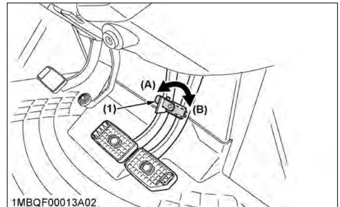
(1) Brake pedal lock (A) “LOCK” (B) “RELEASE”
