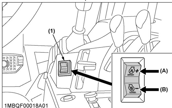
(1) *RPM dual memory switch* (A) *Switch A*
