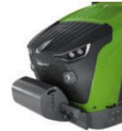
Front weight carrier with 330 kg and slot-in weights with a total of 915 kg
