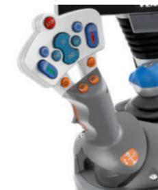
The optional multi-function joystick also features buttons to control two hydraulics valves.
