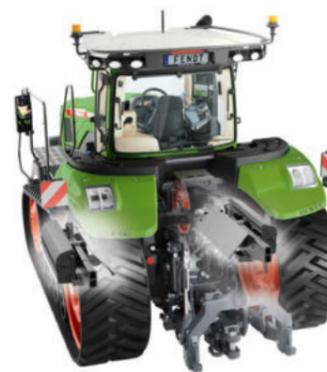
1,345 kg: 32 weights on the outside of the undercarriage (16x per tread); dirt guard on the inside
