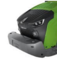
Front weight carrier with 330 kg and single block with 2,000 kg
