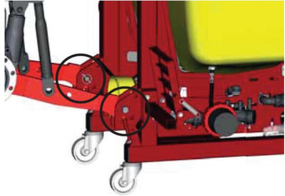
28) Attach the adjustable upper arm of the tractor to the appropriate level of the upper suspension points on the machine chassis and attach the safety pin. **(Figure 8)**
