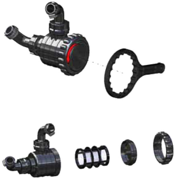
Figure 60 Tank Outlet Filter Removal
