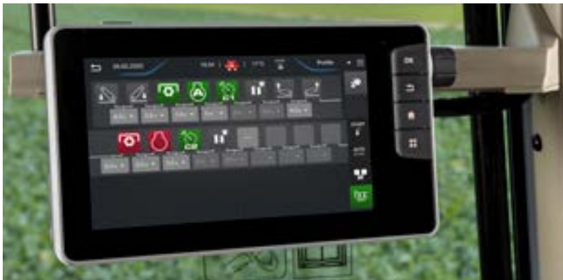
HEADLAND MANAGEMENT is available via the Datatronic (optional on Efficient version).
