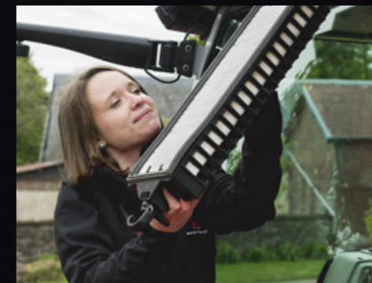
Easy access to remove the cab air filter for cleaning.
