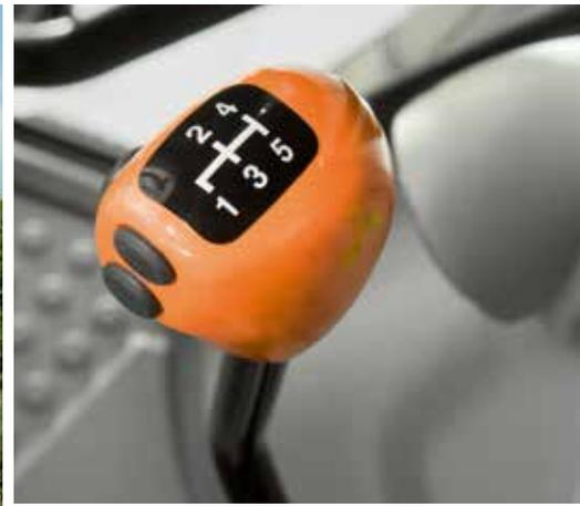
The Powershift stages are shifted conveniently with the press of a button in the shifting lever.
