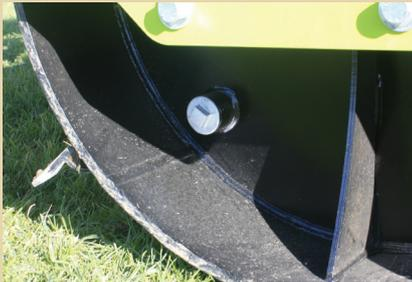
The drum can be filled with water for extra weight to help with ground penetration.
