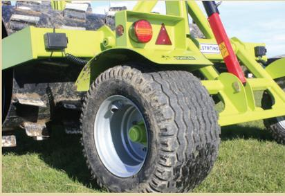
Wide profile flotation tyres, mudguards and LED lights are standard on trailing machines.
