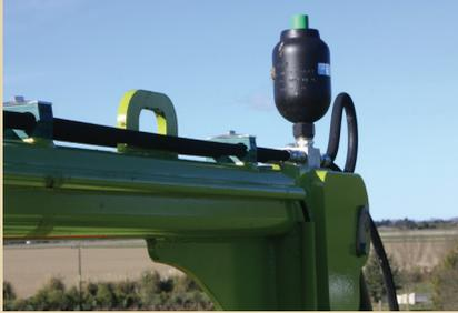
Hydraulic soft ride on the top of the machine for dampening the hydraulics during road transport.
