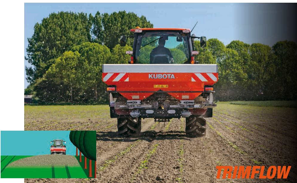
Border spreading from the tramline
