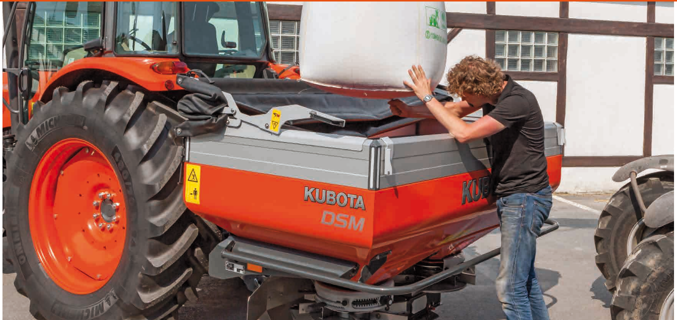
Hopper cover and aluminium hopper extensions
