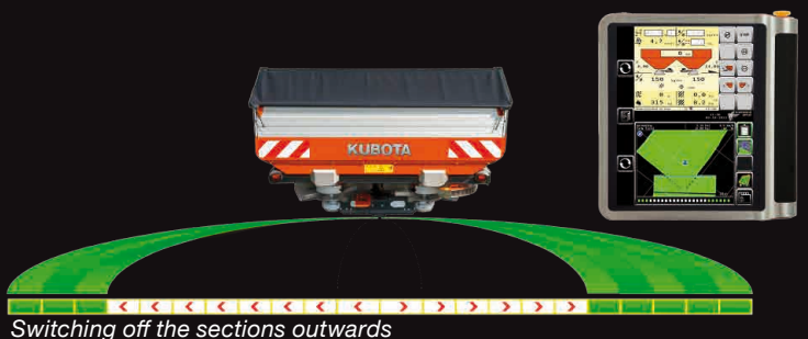
Switching off the sections outwards
