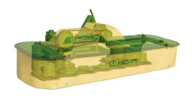
functionality. The compact and light mower is pushed over the surface. Suspended by a pivoting headstock in its centre of gravity and close to the tractor's front wheels, the unit benefits from very little travel to produce perfect cuts, fast crop re-growth and uncontaminated forage.
