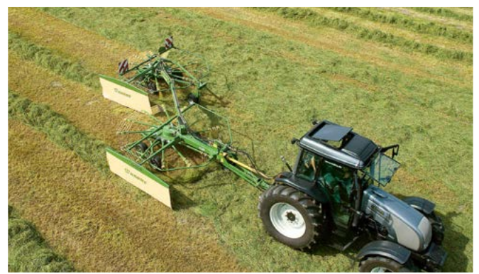
Swadro 710/26 T are the flexible side delivery rakes that produce single and double swaths as well as two swaths.
