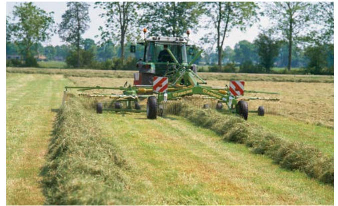
Swadro 810 The side-delivery rake with transport running gear forms single and double swaths as well as two swaths.
