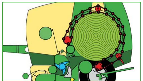
Fixed bale chamber (F 1250): The fully enclosed bale chamber with its endless chain elevator provides for high densities and avoids fragmentation.
