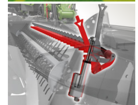
Electric motor steplessly controls the counter comb of the conditioner, which is responsible for the intensity of the conditioning process
