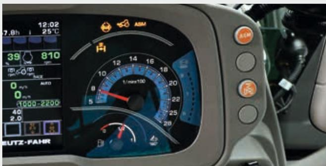
↑ ASM and front axle suspension activation.
