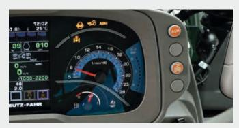
ASM and front axle suspension activation
