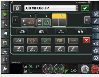
Comfortip further increases the level of comfort. It allows recording of repetitive tasks and their recalling by pressing a single button.
