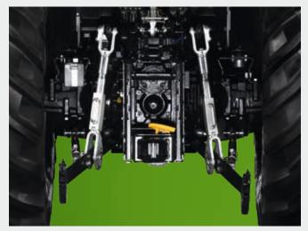
↑ Standard three-point hitch for higher lifting capacity.
