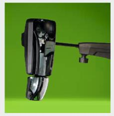
↑ Mirrors with electric adjustment and defrosting.
