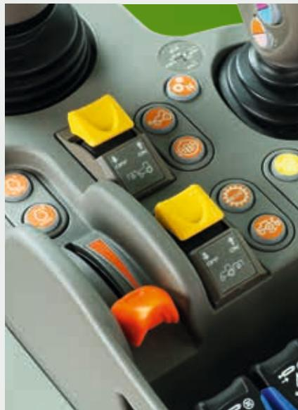
↑ Easy engagement of front and rear PTO through buttons on MaxCom armrest.
