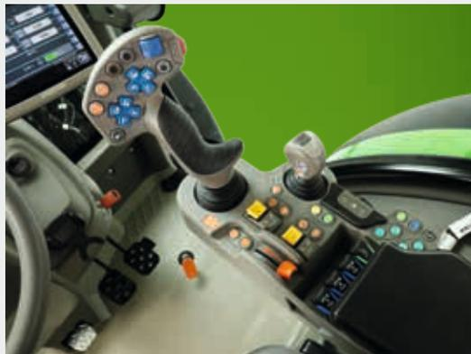
↑ Spool valve easily controlled by joystick and fingertip.
