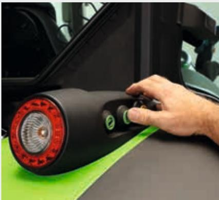
↑ Rear lift and PTO have external controls on rear mudguards.
