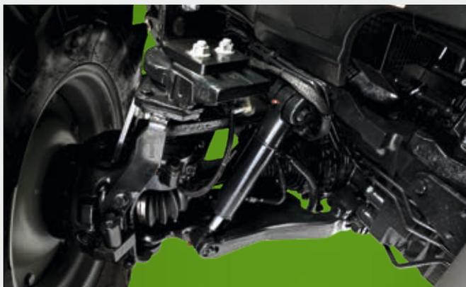
↑ Suspended front axle with front brakes.
