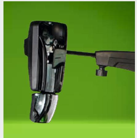
↑ Mirrors with electric adjustment and defrosting.
