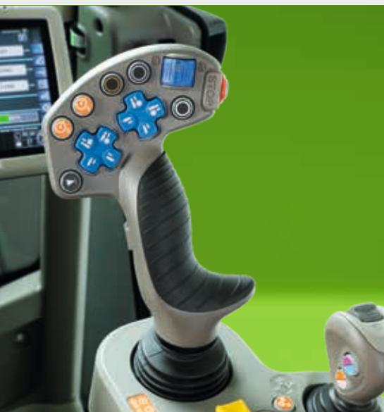
↑ MaxCom joystick for simple management of TTV transmission.
