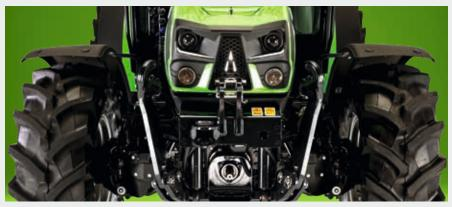
5D TTV models can be equipped with a front lift with 2,880 kg capacity and optional comfort package.
