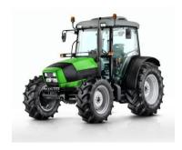
SDF 1000 Series Diesel Engine 4 Cyl/4000cc Turbocharged Liquid/Oil Cooled Bosch High pressure Individual Diesel injection 96Hp @ 2350rpm (2005/25/CE) Torque 342nm Side Mounted Cabin Exhaust 160lt Fuel Capacity
