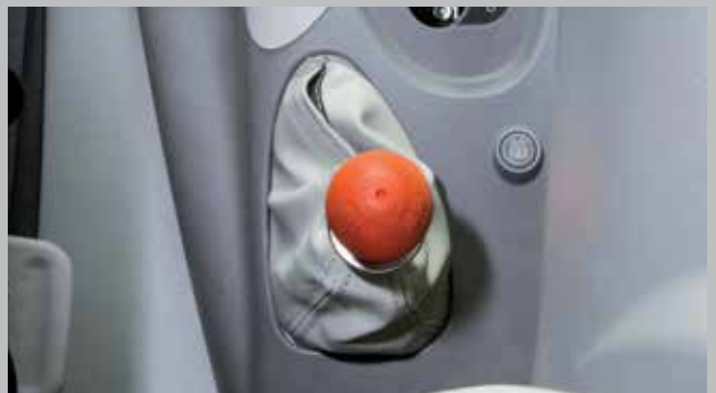
Hydraulic parking brake. A secure position wherever you park your new 6 Series tractor.
