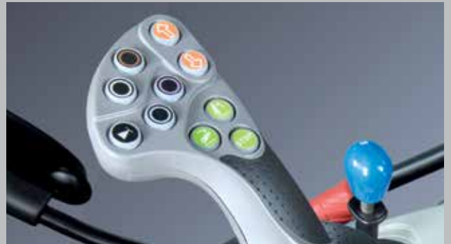
The TTV models are operated using the new PowerCom S joystick. Three buttons can be assigned to any function.
