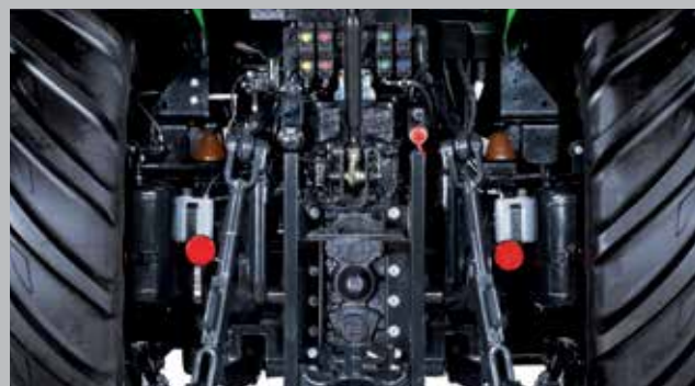
Impressive characteristics: a lifting capacity of up to 7,000 kg and Category II hook ends.
