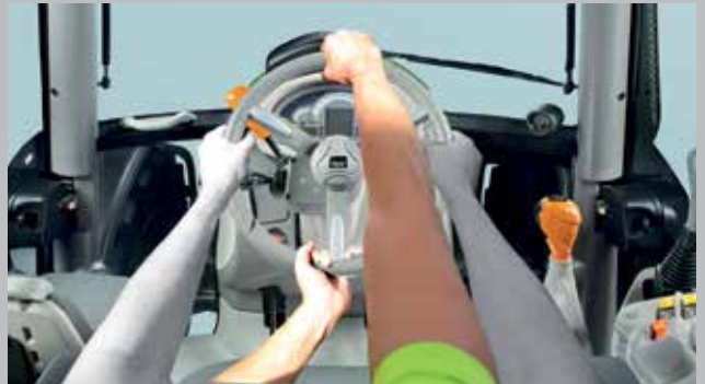
SDD Steering reducing revolutions of steering wheel to two and a half turns to go from one lot to the next.
