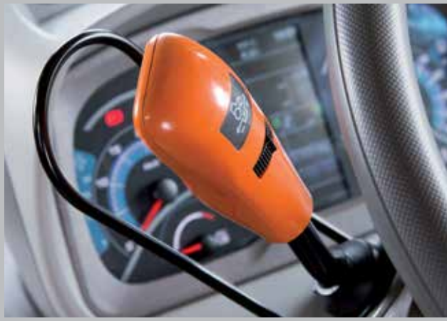
Electro-hydraulic Powershuttle Sense Clutch with modulation for precise and safe changes of direction while driving and with load without interruption of torque.
