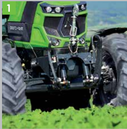
1 Hydraulic packages with 22 equipment options, e.g. a front linkage with ComfortPack.
