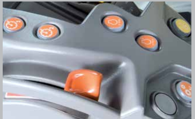
2 Speed engine programming function allowing the operator to set and retrieve desired RPM
