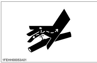
Hydraulic fluid escaping from pinholes may be invisible. Do not use hands to search for suspected leaks. Use a piece of cardboard or wood. KUBOTA also highly recommends use of safety goggles or other eye protection. If injured by escaping hydraulic fluid, see a medical doctor at once. Hydraulic fluid will produce gangrene or severe allergic reaction.
