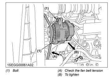
Replace the fan belt if it is damaged.
