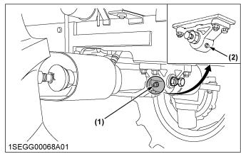
(1) Grease fitting (forward front axle support)
