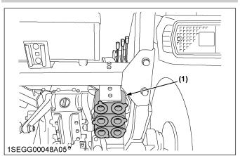
(1) Remote control valve coupler (if equipped)
