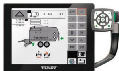
Parallel operation via control lever transfer, Varioterminal and Tigo-Terminal (option)
