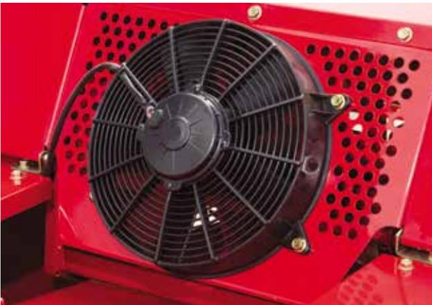
An electric knotter fan is fitted as standard to the MF1840 and ensures the knotters are kept clean and free from any debris build up during operation.
