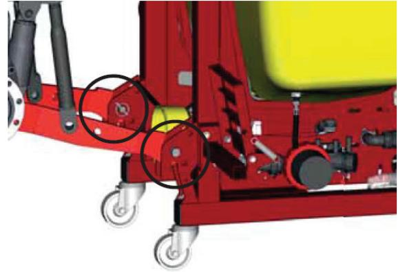
28) Attach the adjustable upper arm of the tractor to the appropriate level of the upper suspension points on the machine chassis and attach the safety pin. **(Figure 8)**
