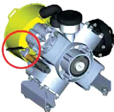
5. Make sure that the by-pass of regulator is in the regulator input lever position. (Figure 35 For Optional FPR Control).
