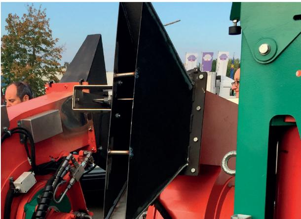
The inclination angle of the blowers can be adjusted and adapted to the row width.
