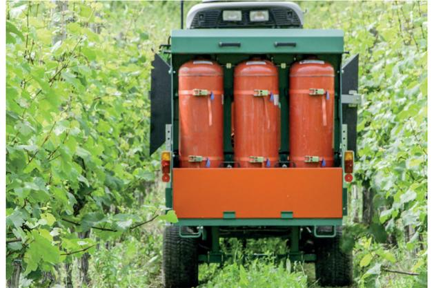
3 different type of gas containers: „EU“, „US“ and „US small“. Gas tank frames and the amount of containers are developed for extended operating time.
