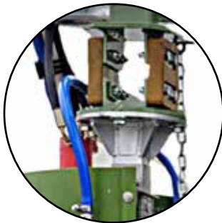
ATTACHMENT OF FANS Flexible pendulum suspension
