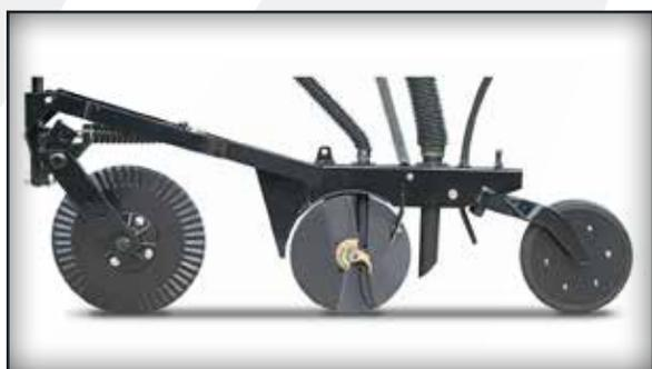
The 06 Series Row Unit by Great Plains utilizes the "Fluff and Plant" no-till system with an integrally mounted coulters to cut residue and prepare a mini-seedbed for the trailing double disc opener. Opener discs are 13.5" (34cm) in diameter with 4mm thick blades, 205 triple-lip sealed bearings, and 1/4" (19mm) opener disc lead.
