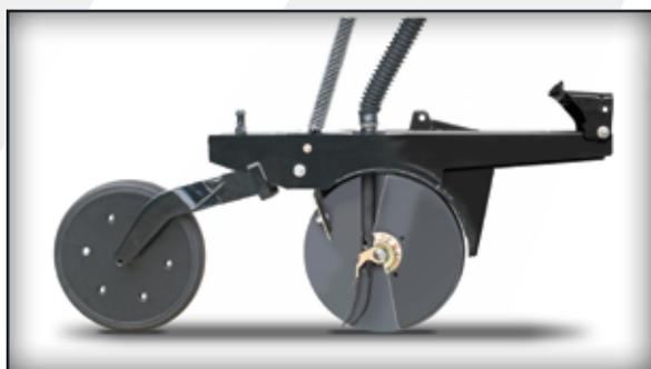
Great Plains 00 Series Openers are designed for min-till fluted feed drills. The 00 Opener features 13.5" (34cm), 4mm blades mounted on 205 triple-lip sealed bearings. The 00 Opener has a 1/4" (6mm) leading opener blade to help cut through tough residue. A rear gauge wheel uses a T-handle adjuster to provide 18 depth-control settings.
